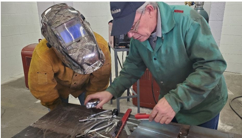
NCTA student Trevor Muellenberg, North Platte, watches Certified Welding Instructor Chuck Hatzenbuehler measure a weld during a certification test administered by the American Welding Society. (Crawford / NCTA photo)
